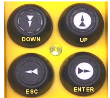
Figure 9 Pushbutton as a Key board for Crane Condition Monitoring Unit
