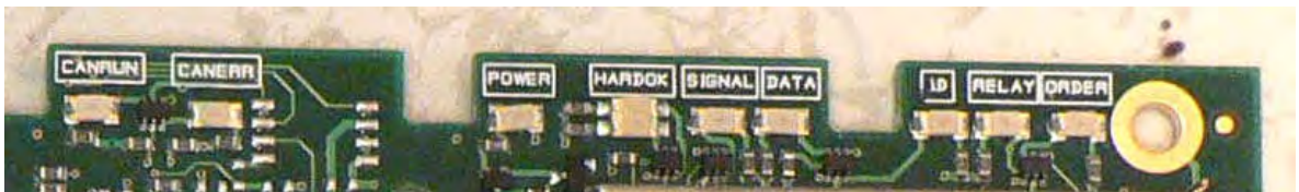
Figure 7. Signalling LEDs in the receiver.
