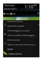
Click the option, switch into USB storage status, at this time the users can access the moveable disk, at the status of USB storage, click the icon again to interrupt USB connect and recover charge mode. USB storage mode system will limit the users use, after interrupt USB storage mode, it will recover into normal status:
