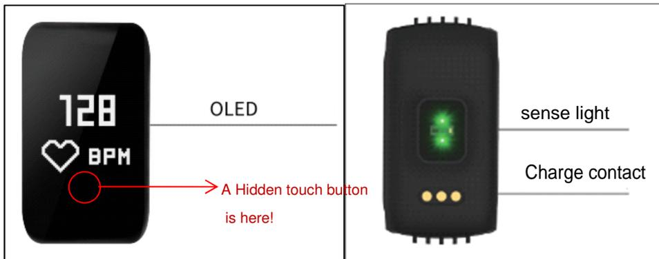
Please ensure the device is full charged for the first time use, you need charge it by charging clip if the device can't power on.
