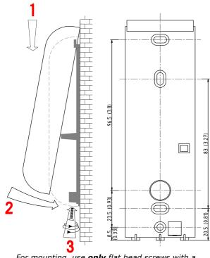
For mounting, use **only** flat head screws with a maximum shank size of 4 mm (5/32", #7)
