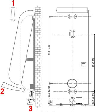
For mounting, use **only** flat head screws with a maximum shank size of 4 mm (5/32", #7)
