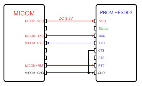
au When TTL level of MICOM is 5V
