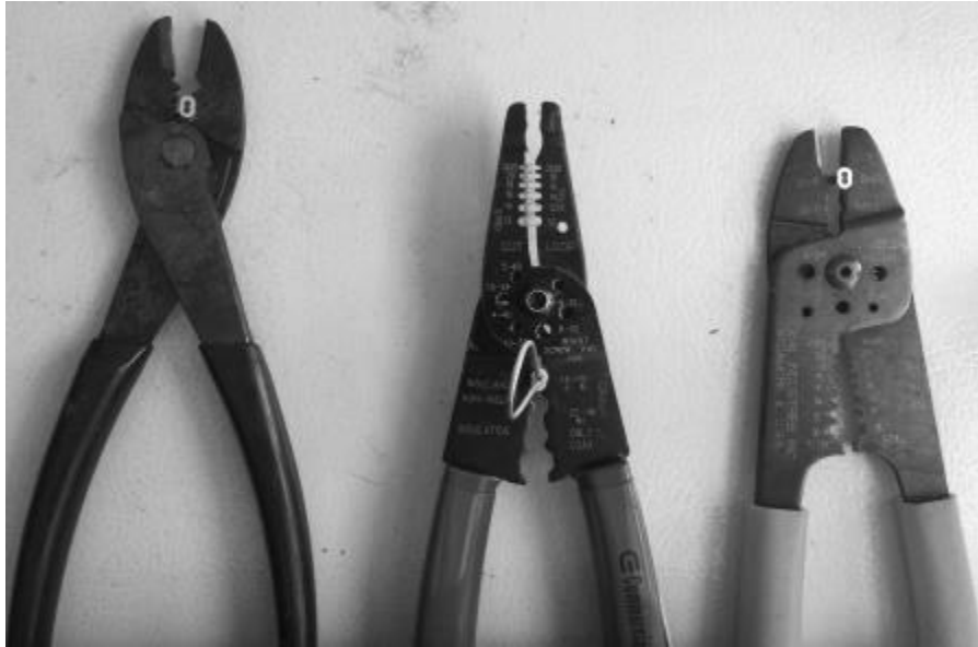
DIFFERENT TYPES OF PLIERS THAT CAN BE USED - SHOWS THE FERRULES IN EACH PLIER TYPE
