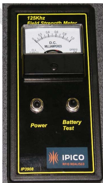
Figure 16: Field strength meter
