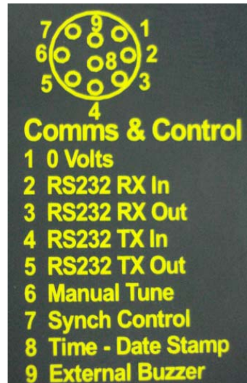
Figure 9: Communications & controls connector pins
