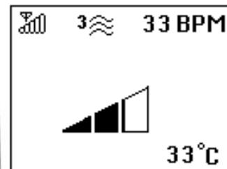
The volume indication bars will pop up on the LCD display when adjusting the volume.
