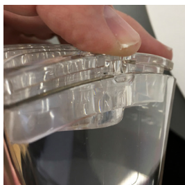
Diffuser plate snaps into place
