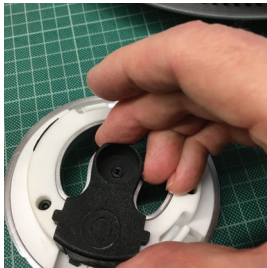
Remove the connector cover.
