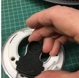
Replace the connector cover.
