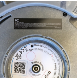
The location of the compliance statements on Atem Purifier is found under the Back Plate cover.
