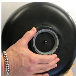
To unlock turn the locking ring.
