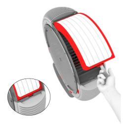
Step 4 Remove the used filter
