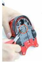
2. Pull out the pin using Long-nose easily
