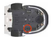
⑥Turn on the switch on the bottom of the robot.
