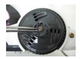
(2) Remove the damaged tire on the wheel and set new tire.
