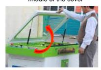
⑤ Pull up until the shock-up pull out fully
