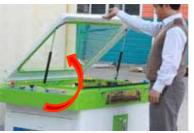
⑤Pull up until the shock-up pull out fully.
