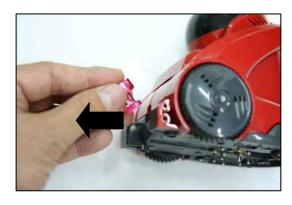
5. Lifting the magnetic ball holder, pull it out to the front.
