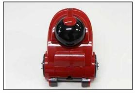
6. The shape after separating a magnetic ball holder from the robot
