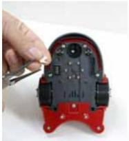
Before taking out the pin using Long–nose, cover the pin by cloth or tissue
