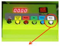
Push the blow button on the control panel.
