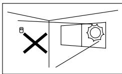
Do not install where the detector is in or facing direct/reflected sunlight, window onto main road to avoid car head light.
