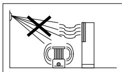
The detector should not face to the ventilation of HVAC or any equipment that may produce strong temperature change.
