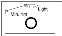
Locate the detector at least 1 meter away from the nearest fluorescent light to avoid interference to MW sensor.
