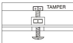
The tamper protection will be activated if the locking screw of front cover and bottom case is loosen. Ensure to fix the screw.
