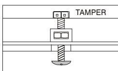
The tamper protection will be activated if the locking screw of front cover and bottom case is loosen. Ensure to fix the screw.
