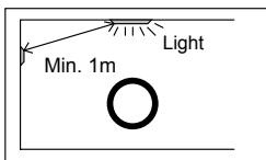
Locate the detector at least 1 meter away from the nearest fluorescent light to avoid interference to MW sensor.
