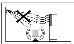
The detector should not face to the ventilation of HVAC or any equipment that may produce strong temperature change.
