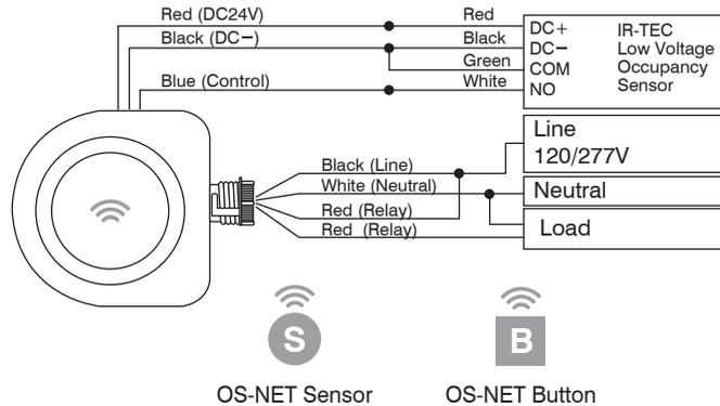
NOTE: For Vacancy Sensing Control (VSC), at least one OS-NET Button should be installed and grouped with the ON-PPU-301 to enable manual-on control.
