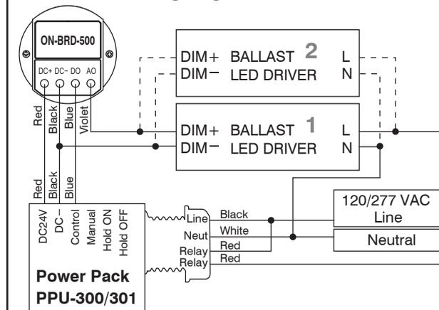
NOTE: Each PPU-300/301 power pack can supply power for up to 2 ON-BRD-500 sensors. When more sensors are connected, multiple power packs may be required.
