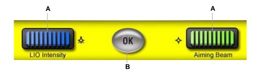
A Displays LIO and Aiming Beam intensity. Use control knobs to adjust.
