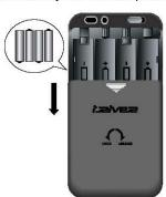
2 Make sure the correct polarity and insert four AA size batteries. Close the cover.
