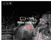
Open the USB cover at the bottom, plug in the USB charging cable, and connect with the power to charge, or use a portable power source to charge the device.
