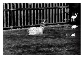
enlarge or **Down button** (8) to reduce the width between the measurement lines, so that the target is completely between the measurement lines. While adjusting the width between the measurement lines, the rangefinding data on the left changes accordingly;
