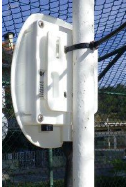
Figure 3 – Example of correct attaching on a gas tank hook with cable ties or glue.
