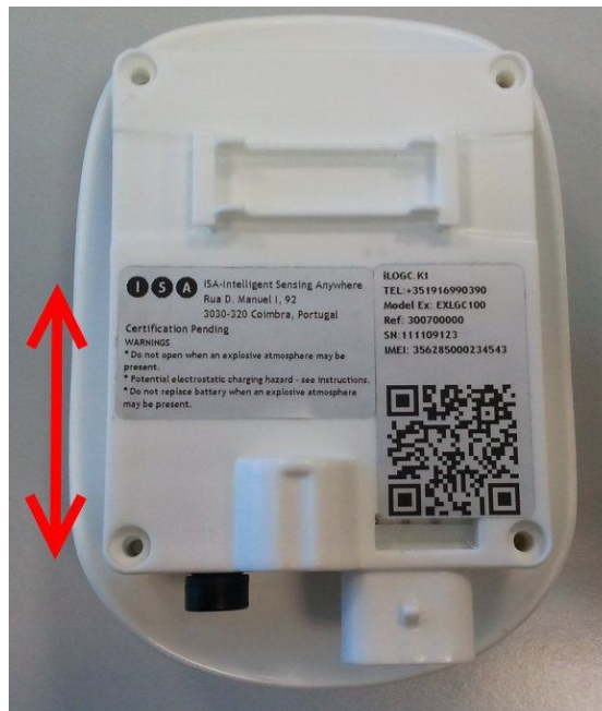
Figure 12 - Location to pass the magnet on the CLOG500 .
