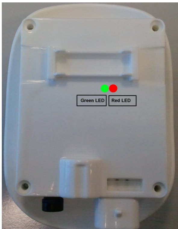
Figure 13 - Location of the red and green LED on the CLOG500 .
