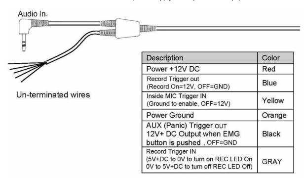
2) Plug the 3.5mm stereo plug into the audio input jack of the recording device.
