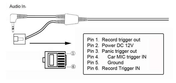
1) Plug the 3.5mm stereo plug into the audio input jack of the recording device.
