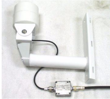
Figure 12. Antenna and Pre-Amp
