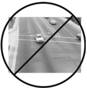
Poor Setup - Stop bar Area Is In The Middle of The Field of View (FOV)
