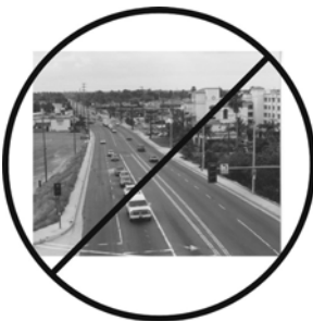
Poor Setup - Horizon Is Included As Part of The Field of View (FOV)
