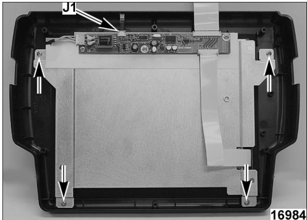
9. Mount RFID board using two screws from kit to secure board to console housing.
