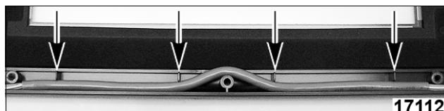
13. Tuck other part of cable with stripped insulation behind post as shown.
