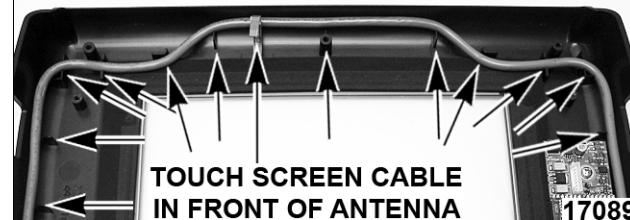
15. Connect antenna cable plug to J1 on RFID board. Dress wires as shown.
