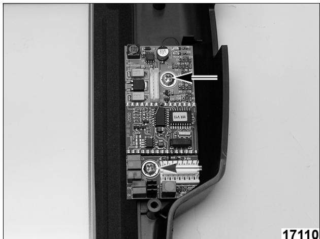
10. Connect antenna cable plug to RFID board J2. Tuck wires behind post as shown and route cable down to corner of housing.
