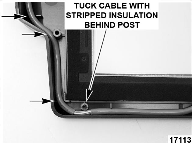
14. Working clockwise, continue to tuck antenna into areas shown. Be sure touch screen ribbon cable is in front of antenna cable.
