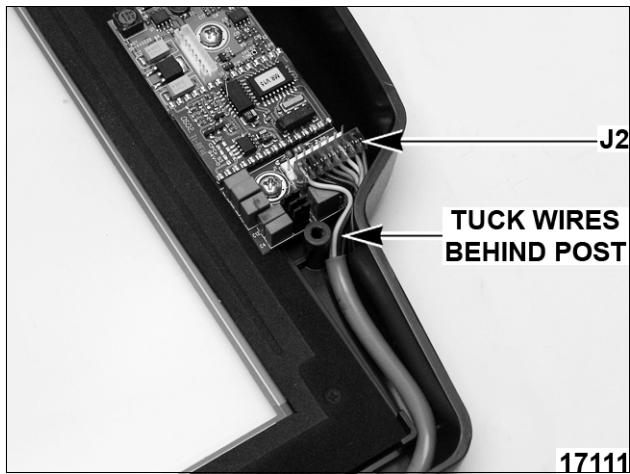
11. Tuck cable with stripped insulation part behind post as shown.
