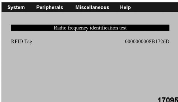
28. When tag is moved out of range, and after a delay, numbers change to all zeros indicating tag is not being sensed.
