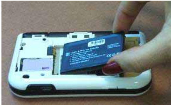
Figure 2: Installing the Battery
