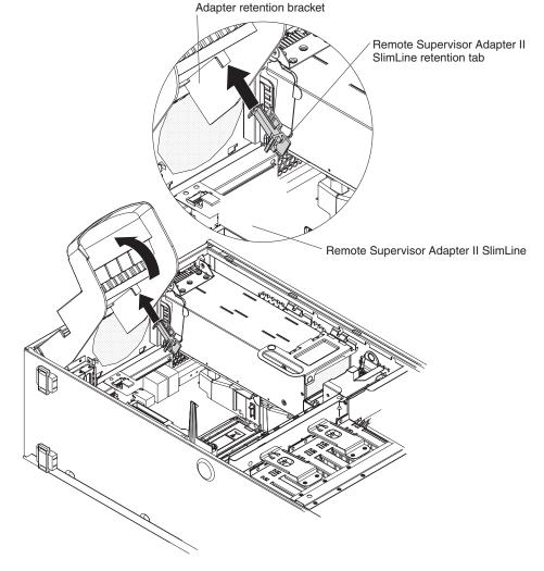
5. Open the rear adapter retention bracket and install the Remote Supervisor Adapter II SlimLine retention tab that comes with the adapter on the bracket by clipping it onto the adapter retention bracket.
