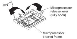
c. Close the microprocessor bracket frame; then, close the microprocessor retention latch and lock it securely in place.
