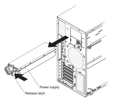
6. Remove the power supply and power supply filler from the server by pressing down on the release latch while you pull out.
