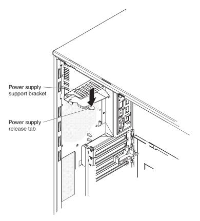
10. Raise the power-supply cage slightly and press and hold the release tab on the rear power-supply support bracket; then, lower the power-supply structure into position. For clarity, the power-supply cage is not shown in the illustration.
