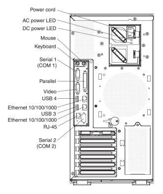
The following illustration shows the connectors and LEDs on the rear of the server.
