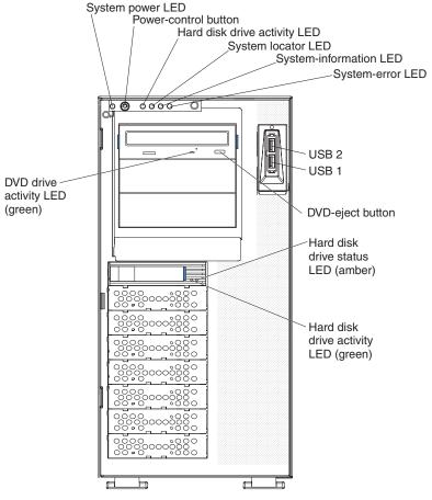
**Note:** The front bezel door is not shown so that the drive bays are visible.
