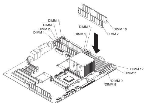
The following illustration shows how to install DIMMs on the system board.
