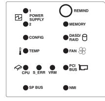
Press the remind button on the light path diagnostics panel to acknowledge that an error has occurred but indicate that you will not take immediate action. When you press the remind button, the system-error LED flashes every 2 seconds until the error is corrected. If another error occurs, the system-error LED stops flashing and is lit again.
