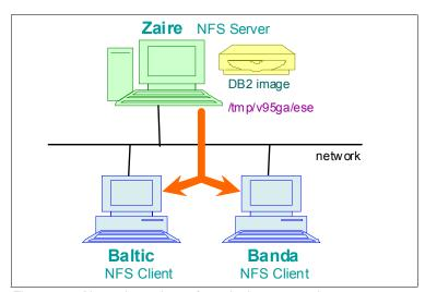
Figure 2-6 Network topology of our deployment environment
