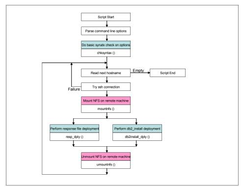
Figure 2-7 Logic of the mass deployment script
