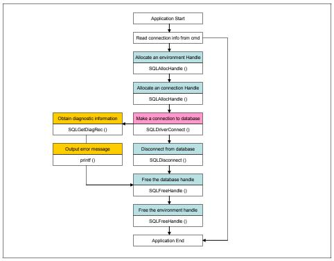
Figure 4-2 logic of sample application
