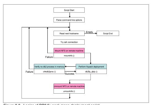
Figure 2-9 Logics of DB2 fix pack mass deployment script
