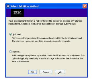
The **Enterprise Management Window Task Assistant** is a series of wizards that helps you install and manage your new DS3000 disk system. The **Task Assistant** helps with common tasks such as:
