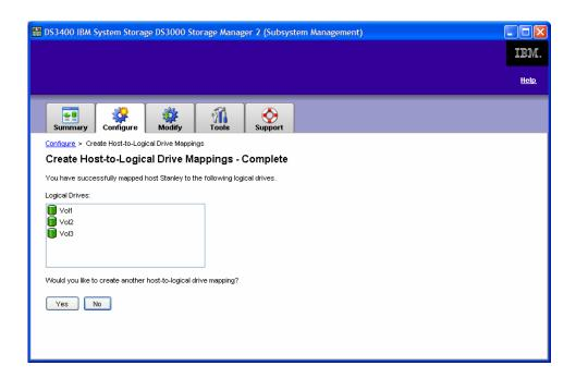
You have successfully created arrays, logical drives and mapped logical drives to a host with the simple Automatic option.
