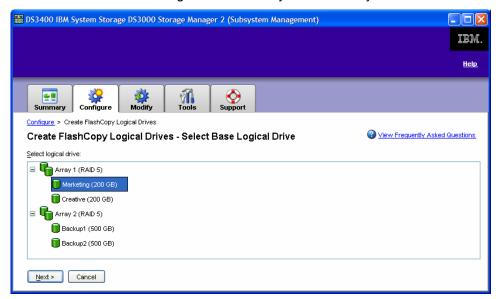
Also note that when you create a FlashCopy logical drive, you automatically create FlashCopy Repository logical drive. A FlashCopy Repository logical drive stores information about the data that has changed since the FlashCopy logical drive was created. Repository logical drives are reserved for DS3000 Storage Manager use. For example, you cannot select a FlashCopy Repository logical drive for use as a base logical drive or as a target logical drive in a FlashCopy or VolumeCopy operation.
