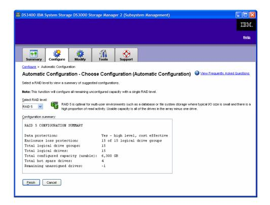
After reviewing your configuration options with RAID 5, return to the task window and select the second step in the Automatic option - **Create Host-to-Logical Drive Mappings**. This will open the **Create Host-to-Logical Drive Mappings** window.
