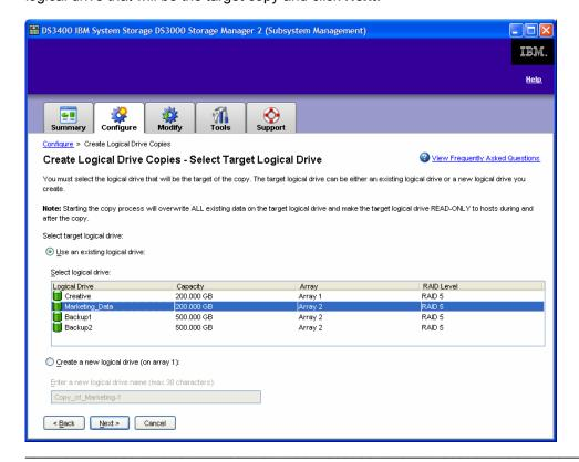
**Note:** Starting the copy process will overwrite all existing data on the target logical drive as well as place the source logical drive READ-ONLY mode during the copy. Therefore, best practice is to copy a FlashCopy image, which will maintain access to the production data.
