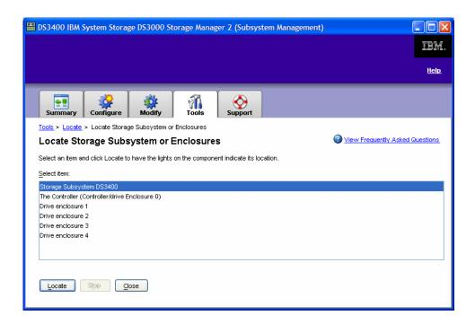
From this screen, select an item and click on **Locate** to have the lights on the DS3000 disk system indicate its location. This allows you to locate the physical location of the disk system in your network. The disk system can then be identified with a label.
