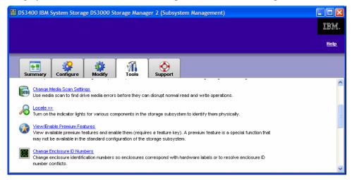
At the **Change Media Scans Settings** dialog box select the logical drives (one or more) to scan and their settings (scan duration and with or without redundancy check). Media scans can also be suspended from this window. Click **OK** and the operation begins.
