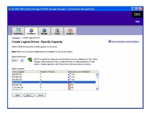
The next window, **Create Logical Drives – Specify Logical Drive**, requires you to select the logical drive capacity from the free capacity that is available, name the logical drive and identify its I/O characteristics. We will select 200GB capacity, name the logical drive **Marketing** and select the I/O characteristics based on a file system application.
