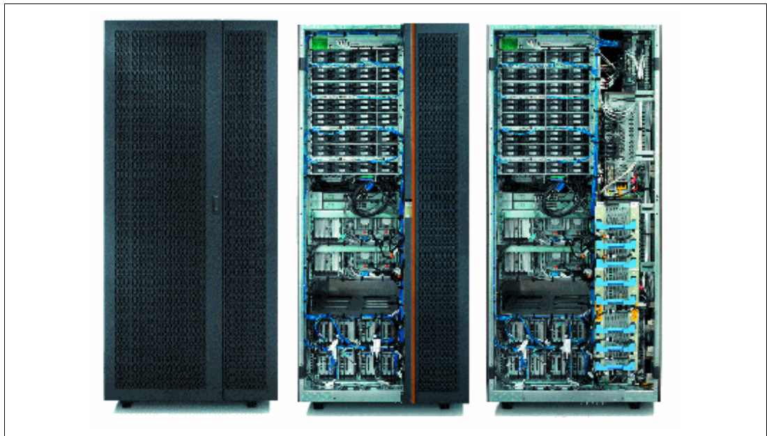
Figure 6-4 DS8300 Model 922/9A2 base frame rear view with and without covers
