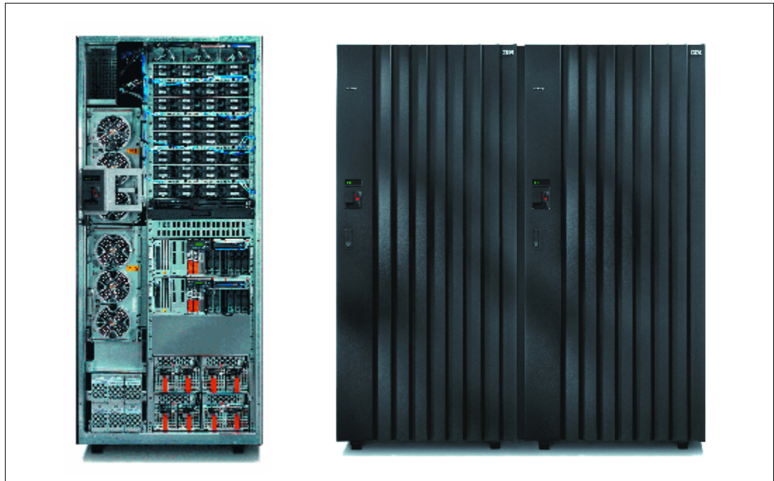
Figure 6-2 DS8100 Model 921 base frame open (left) and with Model 92E for max config
