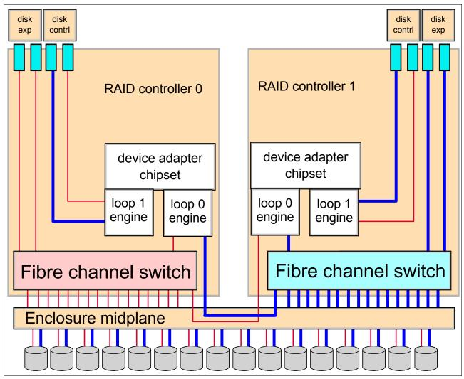
Figure 3-5 DS6000 switched disk connections
