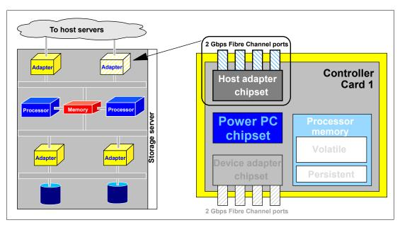
Figure 11-5 Host adapter with 4 Fibre Channel ports
