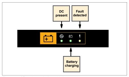
Figure 2-19 DS6000 battery backup unit indicators
