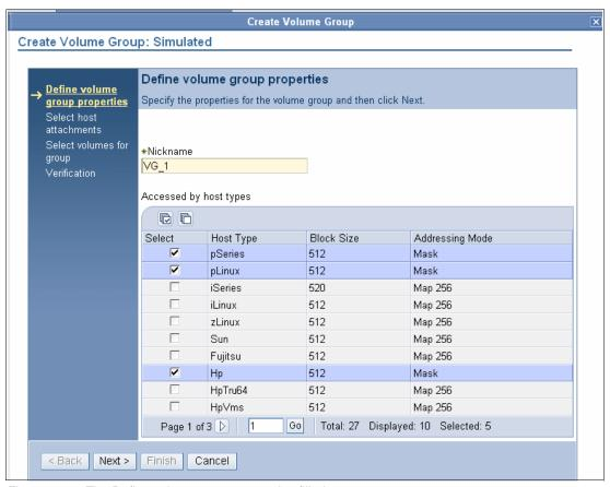
Figure 9-46 The Define volume group properties filled out
