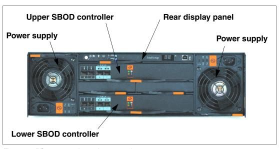
Figure 2-3 DS6000 expansion enclosure rear view
