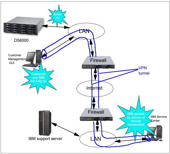
Figure 8-3 DS6000 series configured for remote support
