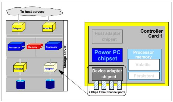
Figure 11-4 Fibre Channel device adapter with 2 Gbps ports
