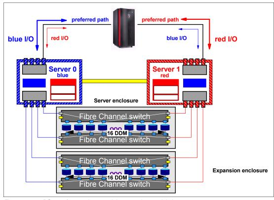
Figure 11-11 DS6800 front end connectivity example - partial view
