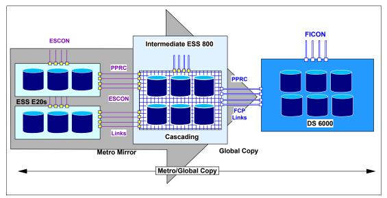
Figure 13-4 Intermediate ESS 800 used to migrate data with PPRC over ESCON
