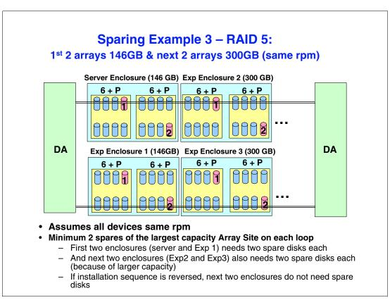
Figure 8-12 Sparing example 3 (add larger capacity DDMs)
