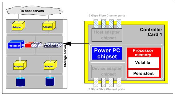
Figure 11-6 Standard PowerPC processor complexes for DS6800-511
