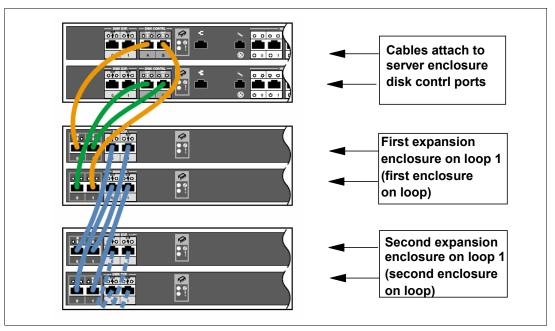
Figure 2-15 Expansion enclosure cabling (Disk Contrl ports on loop 1)
