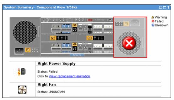
Figure 3-6 Failed power supply
