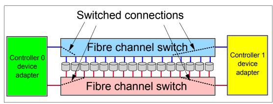
Figure 2-9 Disk enclosure switched connections
