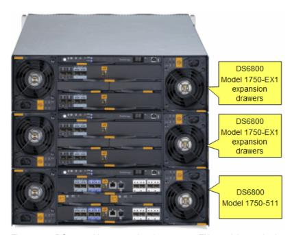
Figure 5-4 DS6000 with 2 expansion drawer 1750-EX1 models attached to 1750-511 controller
