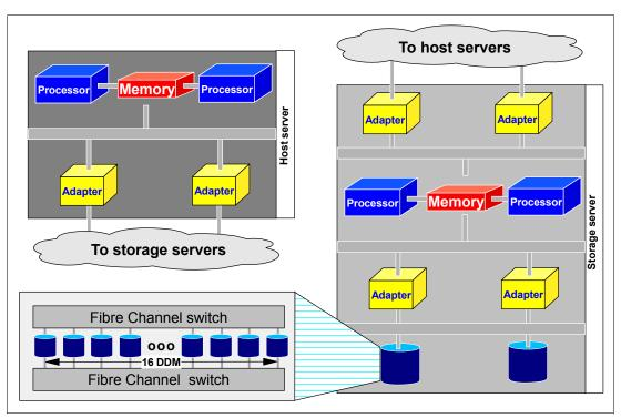
Figure 11-2 Switched FC-AL disk subsystem
