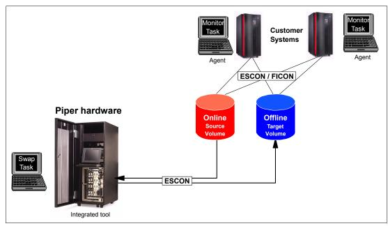
Figure 13-2 Piper for z/OS environment configuration
