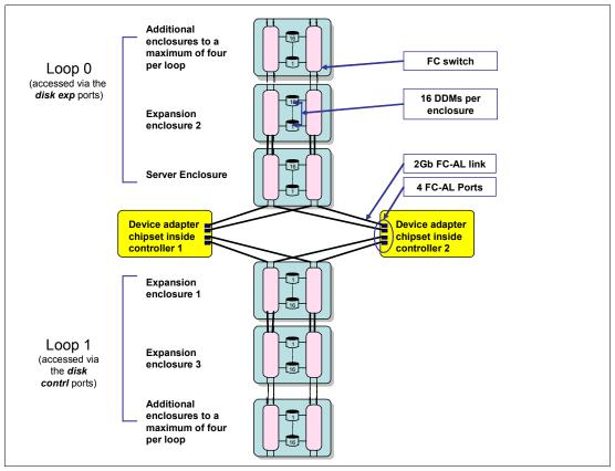
Figure 8-7 Example of connecting several expansion enclosures
