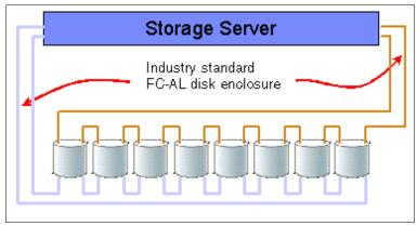
Figure 2-7 Industry standard FC-AL disk enclosure
