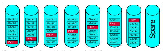
Figure 9-8 Diagram of how parity is striped across physical disks
