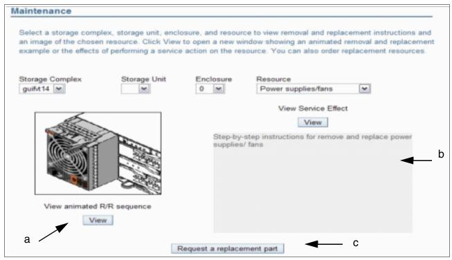
Figure 3-7 Power supply replacement via the GUI
