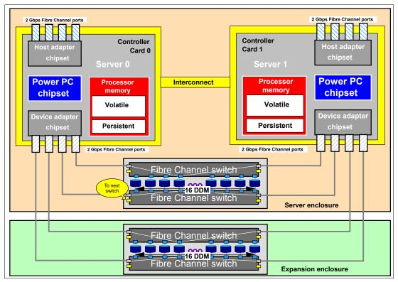
Figure 11-8 DS6800 with one DS6000 expansion enclosure
