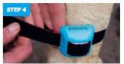
Make sure that the IceQube is positioned with the unique identification number pointing up. There are also arrows on the sides of the IceQube to show the correct way up.
