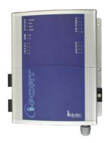
Up to four antennas (plus one extra send antenna) can be connected to i-PORT III. Built-in signal strength measurement capability enables the localization of tags using triangulation.
