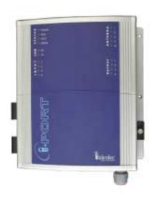
i-PORT3 is the next generation of IDENTEC SOLUTIONS' ILR interrogators. It is capable of communicating not only with tags from the i-Q series, but also with tags from the i-D2 series. The communication range is up to 100 meters for i-Q tags and up to 6 meters for i-D tags.
