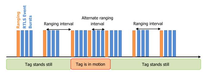
In this mode, the Transponder will broadcast distances measured after the ranging is done. As soon as the Transponder considers it has stopped moving, it resumes its standard behavior.
