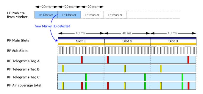
The last row shows how the random use of the timeslot avoids collision between the Transponders.
