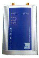
The i-PORT M350-2 is a reader for the i-Q350 and i-B350 series of IDENTEC SOLUTIONS's Response and Broadcast Transponders. Built into a compact housing, the i-PORT M350-2 reads and writes data to the transponders at distances of up to 500 meters (1640 feet) on two antennas. Connection to the host system is established via a RS422 interface, resulting in the capability to connect up to 8 readers in a Daisy Chain using commercially available CAT 5 cables and connectors.
