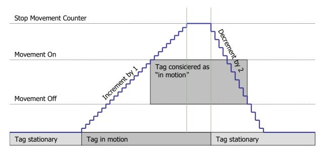
So by adjusting these 5 parameters of the movement counter, short-term influences can be eliminated.
