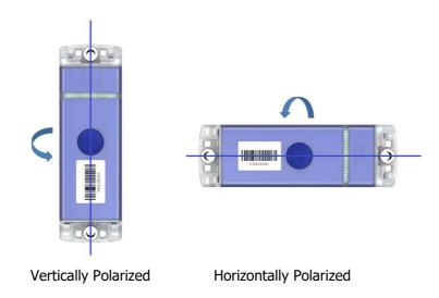
Polarization is dependent on orientation and is rotation symmetrical.
