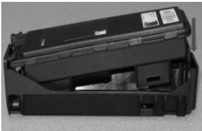
Figure 4.2 Installing the SET transponder into the bracket
