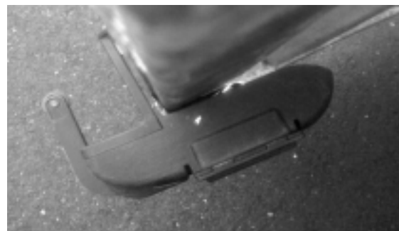
Figure 4.8 CST inside left door mounting
