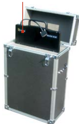
Transport case with temperature control for digital X-ray plate
