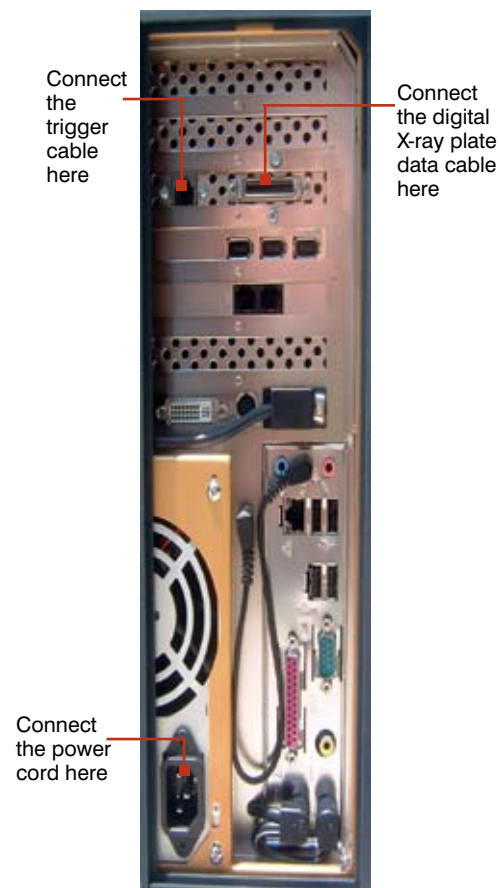
Computer connections for the manual trigger
