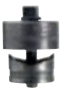
Hole cutter - for drilling the hole for the mixer tap in the sink (35 mm).
