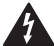
**DANGEROUS VOLTAGE:** The lightning flash with arrowhead, within an equilateral triangle, is intended to alert the user to the presence of uninsulated dangerous voltage within the product's enclosure that may be of sufficient magnitude to constitute a risk of electric shock to persons.
