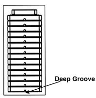
Slide weight plates onto Guide Rod from top to bottom. The deep groove on each weight plate needs to face front and downwards.
