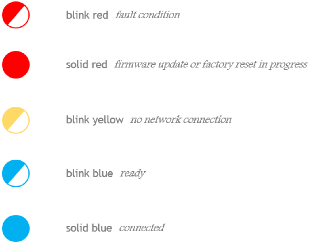
Figure 4.2 LED Light Behavior
