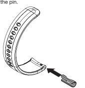
Use the pin removal tool to push in the other side of the pin and pivot the band into place.
