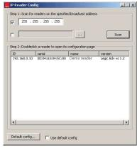
The DHCP server has found the IP Reader and has displayed the host name "PoE Test". The IP-address is also retrieved and displayed.
