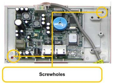
• Use the two self tapping screws to secure the bottom cover to the machine.
