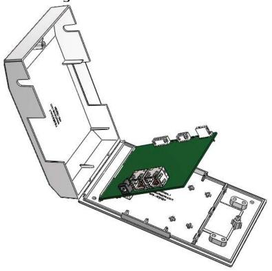
Connect the antenne board to the IP Reader Print board and use the cable clip to secure the cable to the housing.
