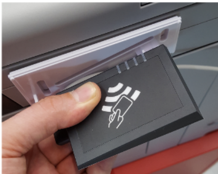
4. Put the reader to the bracket base. Align the cylinders with the holes.
