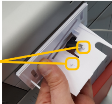
2. Stick the bracket base to the MFP. Make sure to feed the cable through the hole in the bracket.
