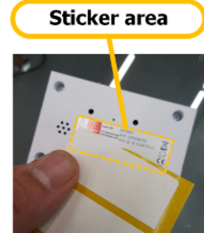
3. Apply the double-sided tape to the reader. Make sure to stay within the serial sticker area!
