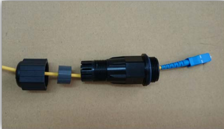
Figure 11 - SFP Connection Step 1
