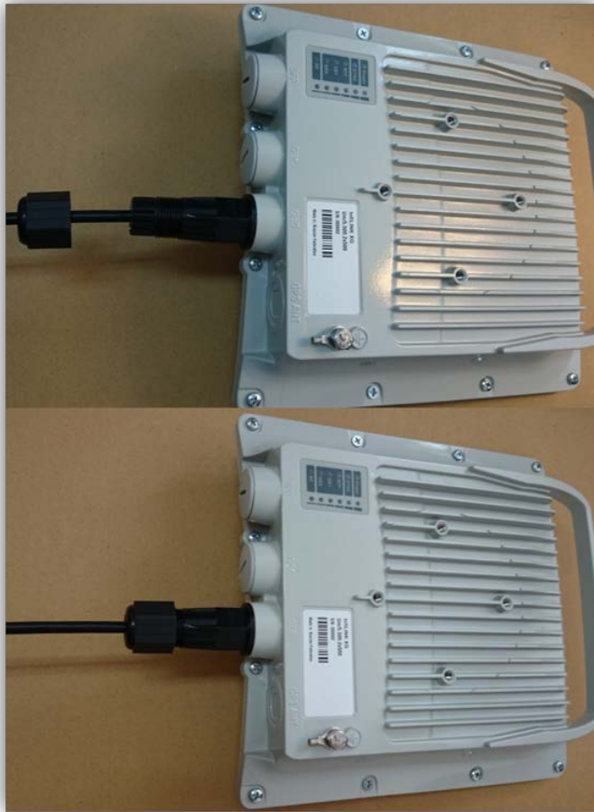
Figure 9 - RJ-45 Connection Step 2
