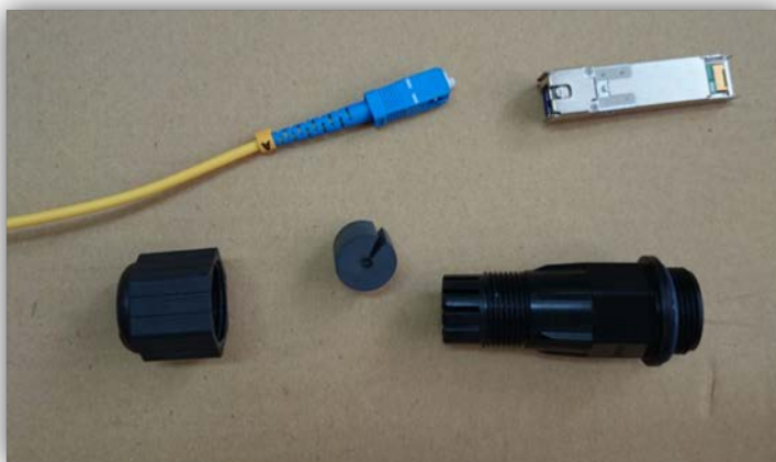
Figure 10 - SFP Connector Components
