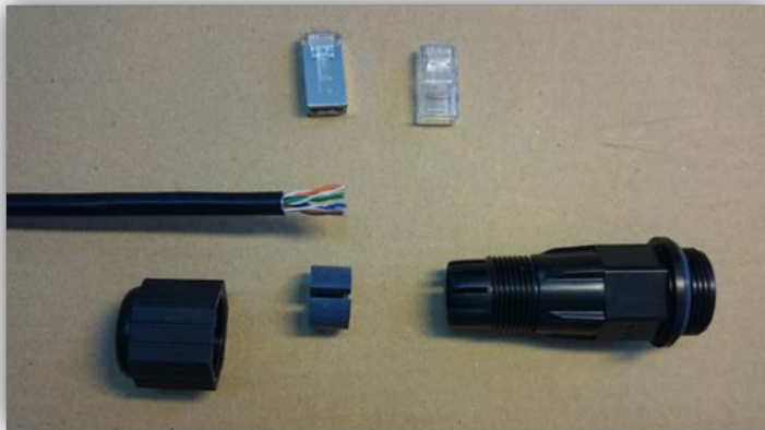
Figure 7 - Ethernet Connector Components
