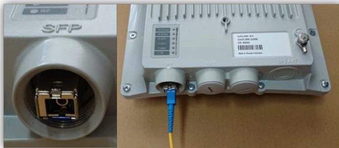
Figure 12 - SFP Connection Step 2
