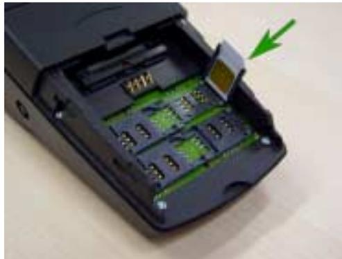
4. You can now close the slot again; the SAM will be positioned towards a plastic stop, which has the same shape as the missing corner. Gently slide the cover back to the right or left, until you hear a small click. The SAM is now firmly attached to the terminal.
