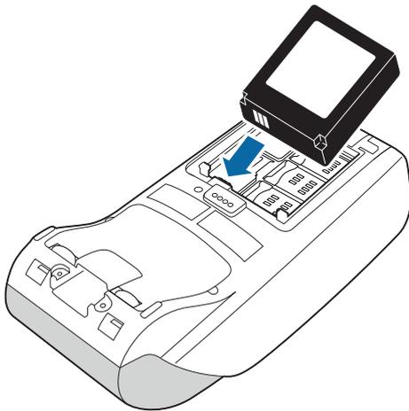
*Figure 14. Inserting the battery*
