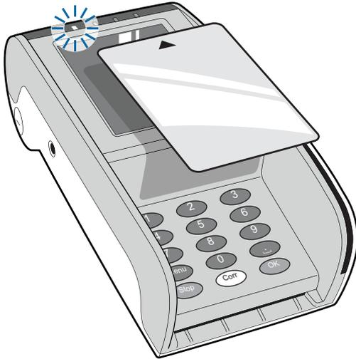
Figure 23. Reading a smart card with the contactless reader
