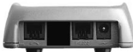
The ELITE 770 terminal must be powered off before connecting the cable on the base, to the RS232 port..
