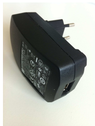
PSU for battery charging
